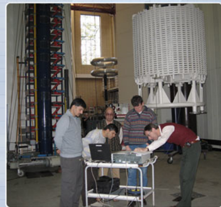
Line trap / 1mH / 2000 A / 50 KA KEMA - high power lab.
